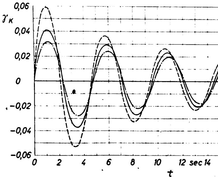
Figure 8. Example: Angle of Inclination of Trajectory for Different Entrained Air Masses; ---  $\mu_K = 0.6$ ; —  $\mu_K = 1.0$ ; - - -  $\mu_K = 1.4$ .
