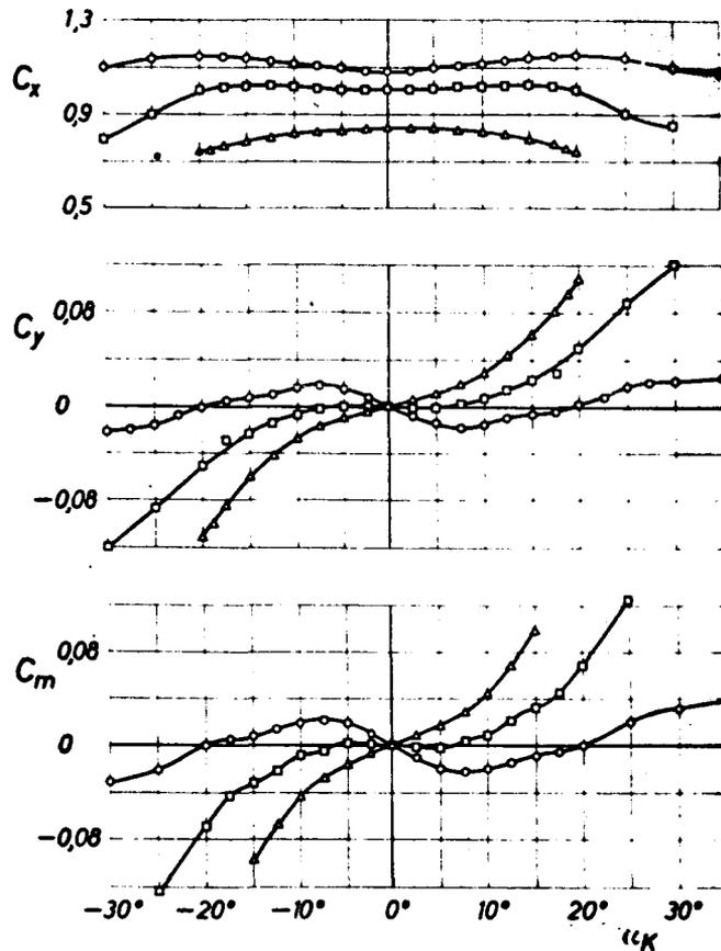
Figure 3. Aerodynamic Values for Personnel Glide Surface Parachute.
